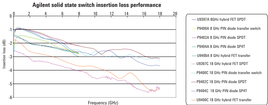
Figure 9. Agilent solid state switches – typical insertion loss performance
